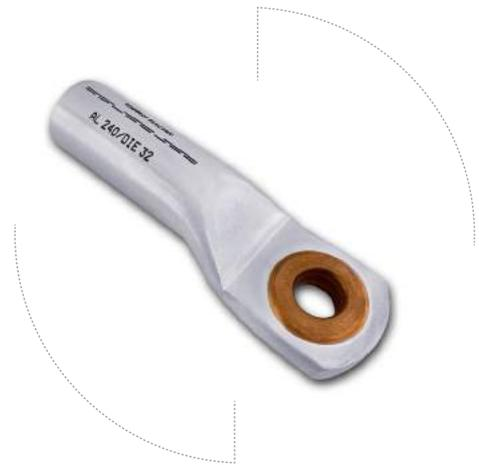
Bi-metallic insert (ring) lugs assure a maximum reliability connection of aluminum cables to copper busbars,copper bushings,..etc.
